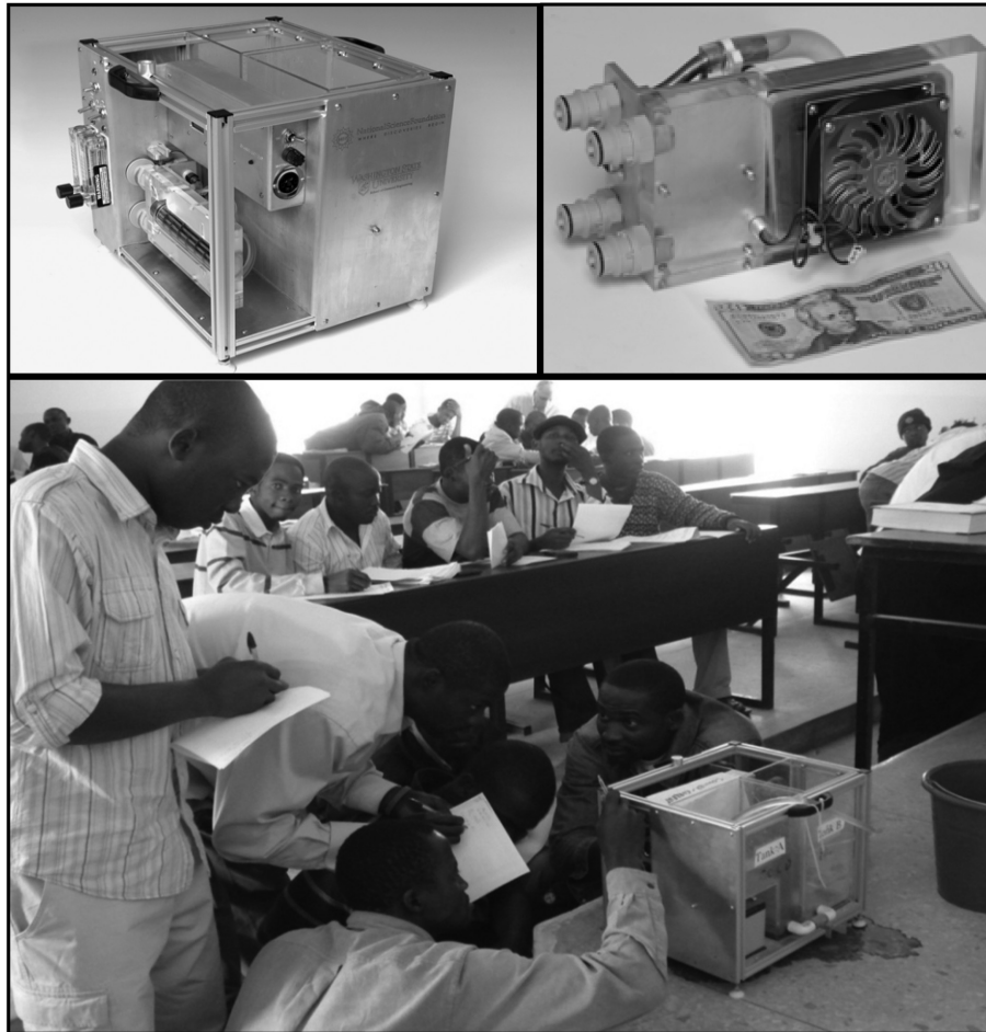
Fig. 1. (a) the DLM with a detachable shell and tube heat exchanger inserted; (b) the extended heat exchanger cartridge used in this study; and (c) a Nigerian HAL classroom with DLMs.
