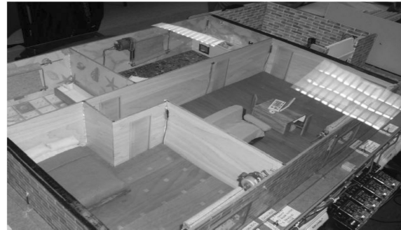
Fig. 4. Scale model prototype. This model is connected with an automatic controller, and this is connected with the graphical interface. The control modes are: automatic, manual.
