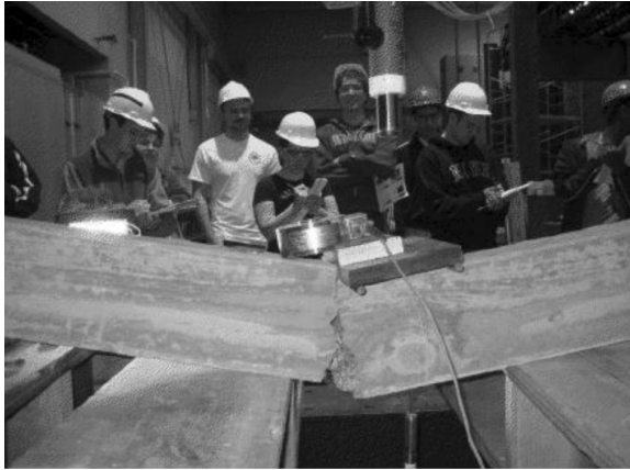
Fig. 2. Students test a concrete beam fabricated using the winning mixture from the impromptu design exercise.
