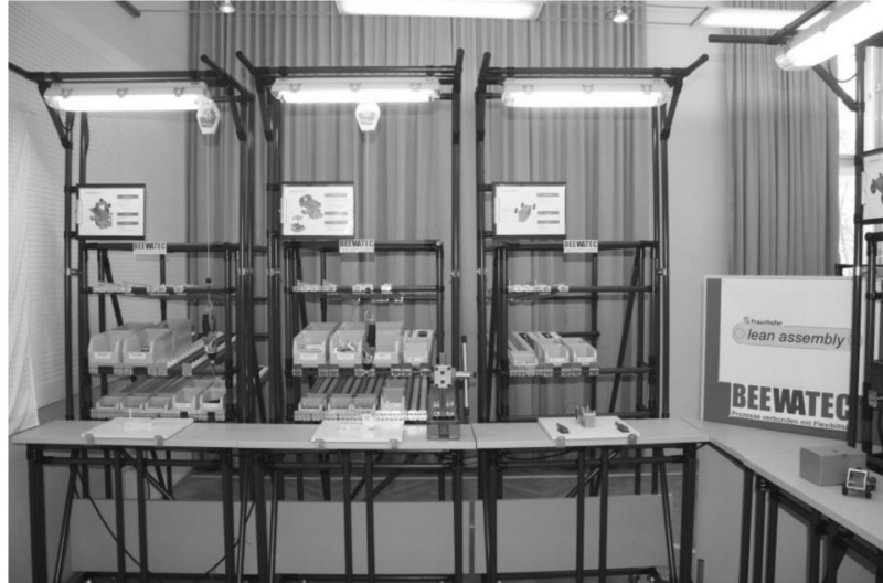
Fig. 5. Assembly line with flexible mounting stations and flow racks.
