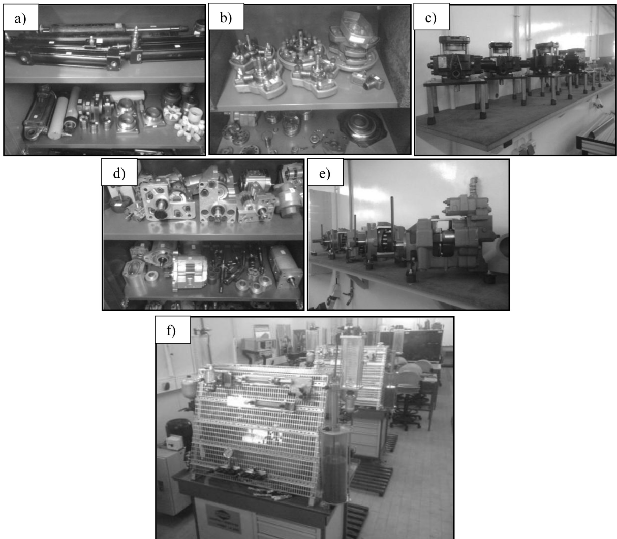
Fig. 6. Some examples of hydraulic components and experimental rigs at the hydraulics: (a) linear actuators and disperse components, (b) radial piston pumps, (c) vane pumps, (d) gear pumps, (e) axial piston pumps (f) experimental test-beds.
