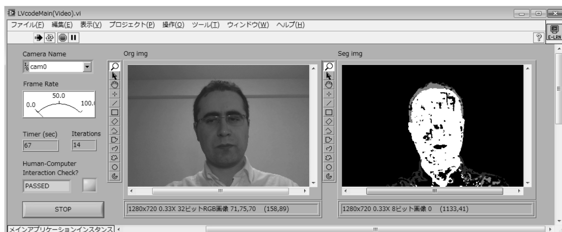
Fig. 7. Front panel of LabVIEW when analysing video frames.
