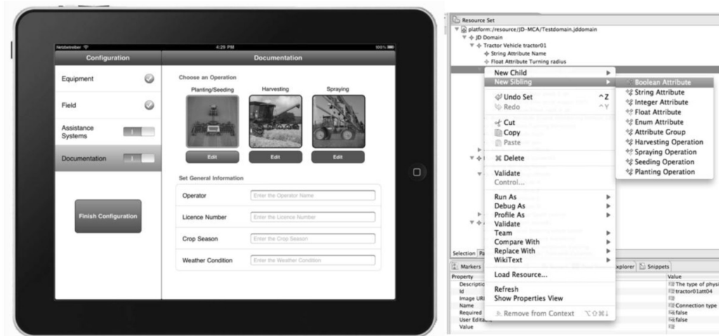
Fig. 3. User interface supporting implement configuration on an iPad and underlying domain model editor.
