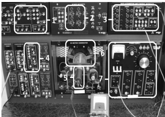
Fig. 5. Power Lab DC motor bench: 1- PID board; 2- Power MOSFETs in an H-bridge configuration (used as a buffer); 3- Data acquisition interface; 4- Chopper/inverter control unit (used to convert analog signal to PWM signal); 5- Tacho-generator; 6- DC motor; and 7- Power supply.
