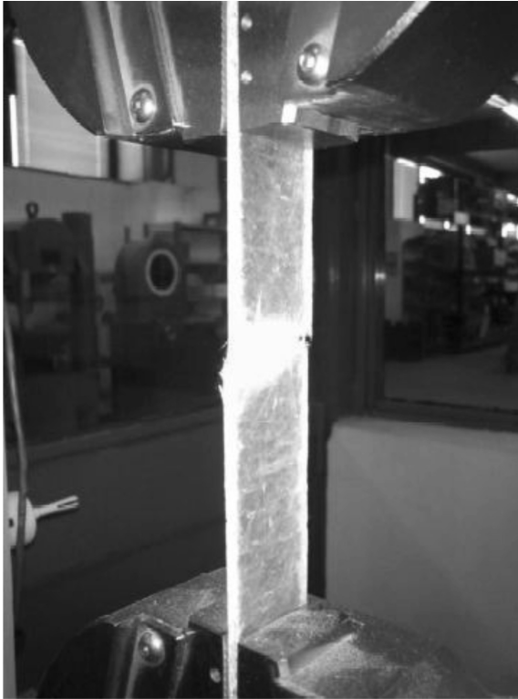
Fig. 1. Tensile test on coupons made from flat polystyrene plate.
