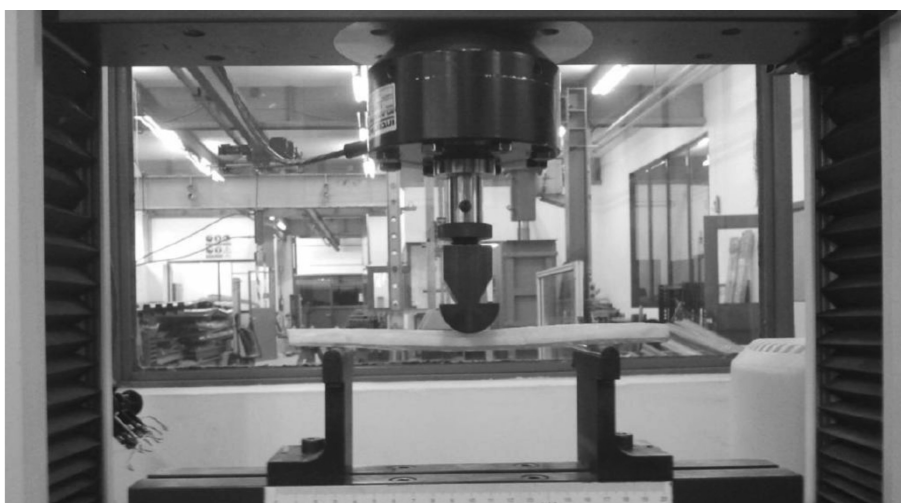
Fig. 3. Flexural test on sandwich panel (three-point bending test).
