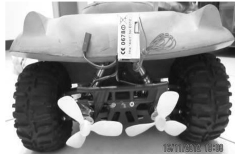
Fig. 5. Two sets of propellers are installed at the back of the boat.
