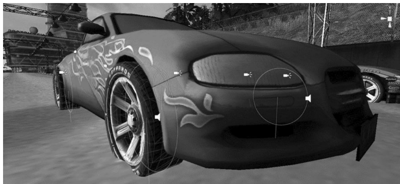
Fig. 3. A screenshot of the wheel colliders (displayed as green rings) on the wheels of a car object.
