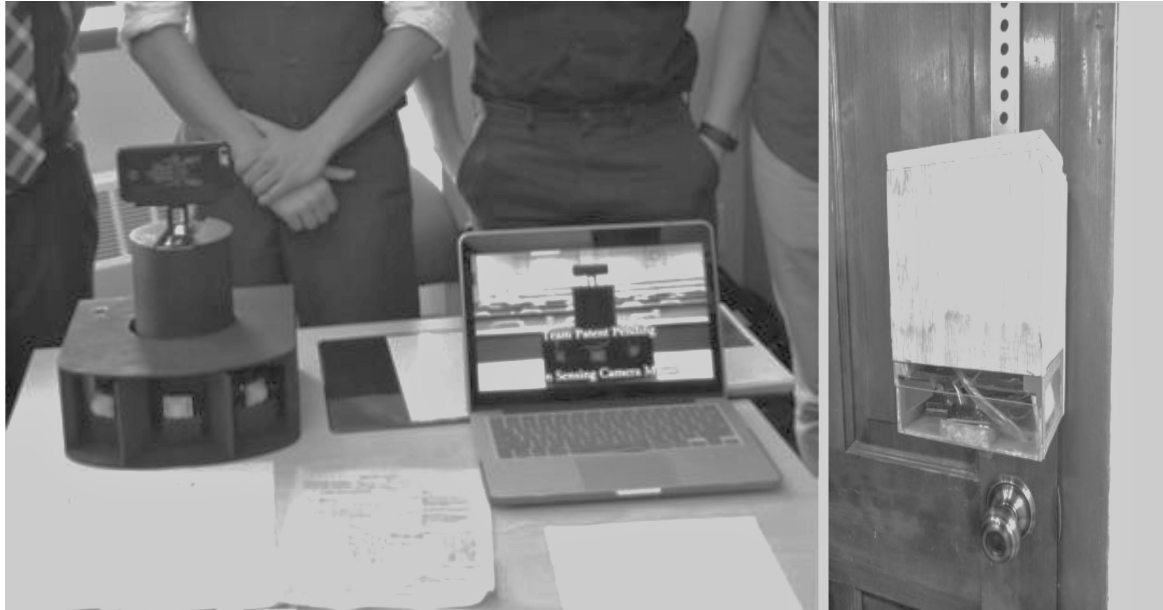
Fig. 2. Examples of mid-program design projects. Left: A motion following camera using a smartphone. The team developed a camera system to track a moving person at the front of a room. Right: Doorknob sanitizing device, inspired by the Covid-19 pandemic. After the door handle was touched a sensor sent a signal to spray disinfectant onto the handle.
