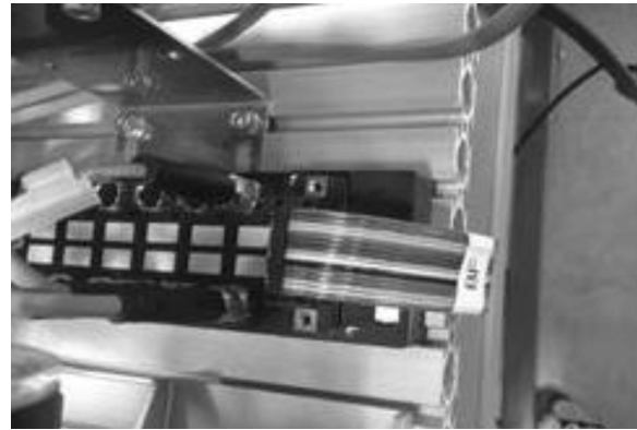
Fig. 10. Ribbon Cable Connections Between Festo Easy Port and Field Devices.
