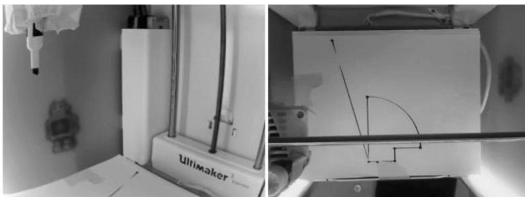
Fig. 4. Remote Views of Printer Head and Completed Drawing After CNC Coding Exercise.
