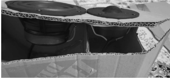
Fig. 3. P14's first working prototype, with portions of the cardboard left untaped to allow for iterative changes.
