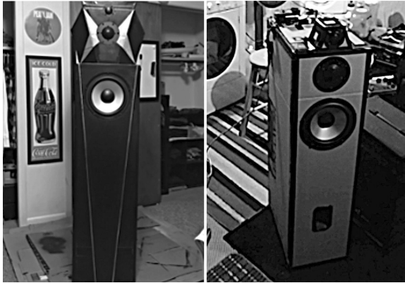
Fig. 1. P1's first working prototype (left) versus final working prototype (right), showing adjustments to enclosure sizing and driver placements.
