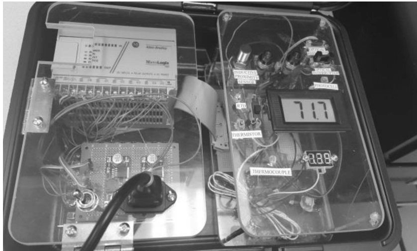
Fig. 3. Portable PLC Kit with Sensor module on the right. The module includes an inductive proximity sensor, resistance temperature detector (RTD), thermistor, thermocouple, optical reflector, optical interrupter, and photocell.
