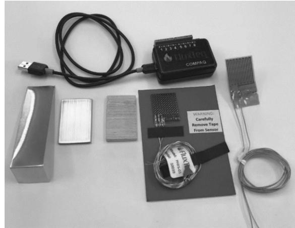
**Fig. 1.** Components of the PEP Heat Transfer System.
