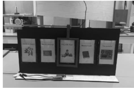
Fig. 4. Sip and puff and light touch switch operable communication board. Project context: Engineering for communication.
