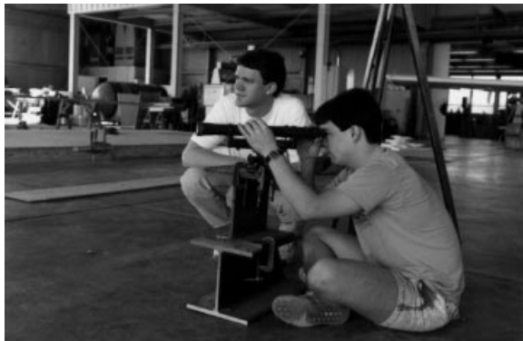
Fig. 14. Transit leveling structure.
