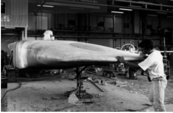
Fig. 24. Canopy and nose applied.
