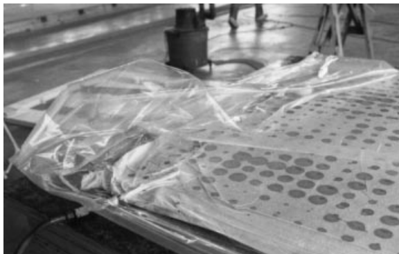
Fig. 19. Vacuum bagged skin panel.
