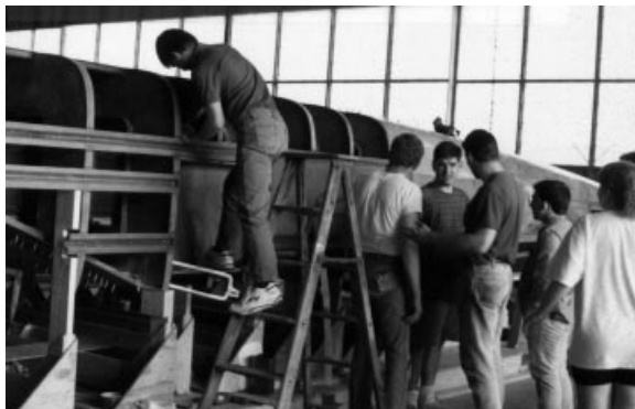
Fig. 20. Applying skin to skeleton.
