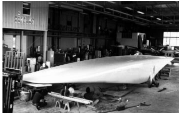
Fig. 28. Base coat of paint applied.
