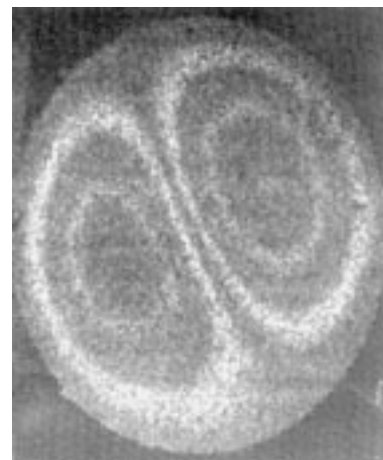
Fig. 4. Time-average fringe pattern of a circular plate with clamped boundary vibrating at its 2 nd resonance.
