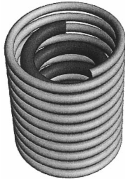
Fig. 3. A pair of concentric springs of minimum outside diameter but of fixed inside diameter, total stiffness and preloaded length.
