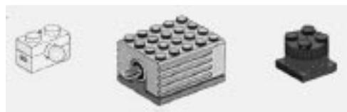
Fig. 2. LEGO output devices.
