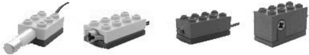
Fig. 3. The LEGO sensors.
