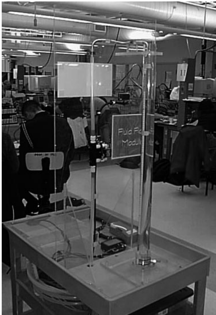
Fig. 2. Fluid Standpipe module in use at a LabStation.
