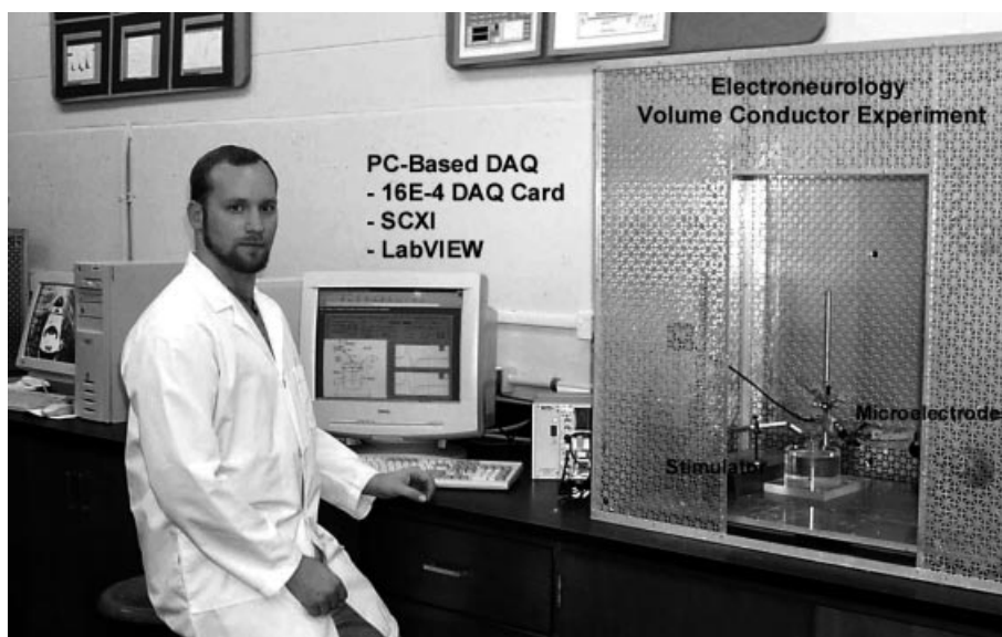
Fig. 1. Typical biomedical systems and instrumentation laboratory workstation. It is shown here configured for an experiment demonstrating the effects of a volume conductor on electroneurology recordings.
