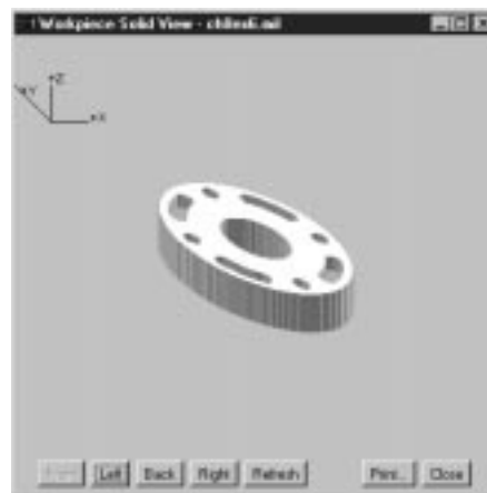
Fig. 4. Aluminum elliptical flange simulation in CNCez.
