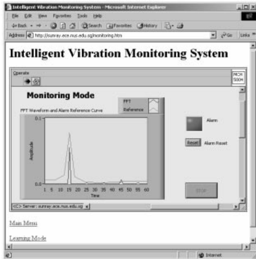
Fig. 10. Snapshot of the interface when the system is in the monitoring mode with the shaker receiving a 15 Hz square wave signal.
