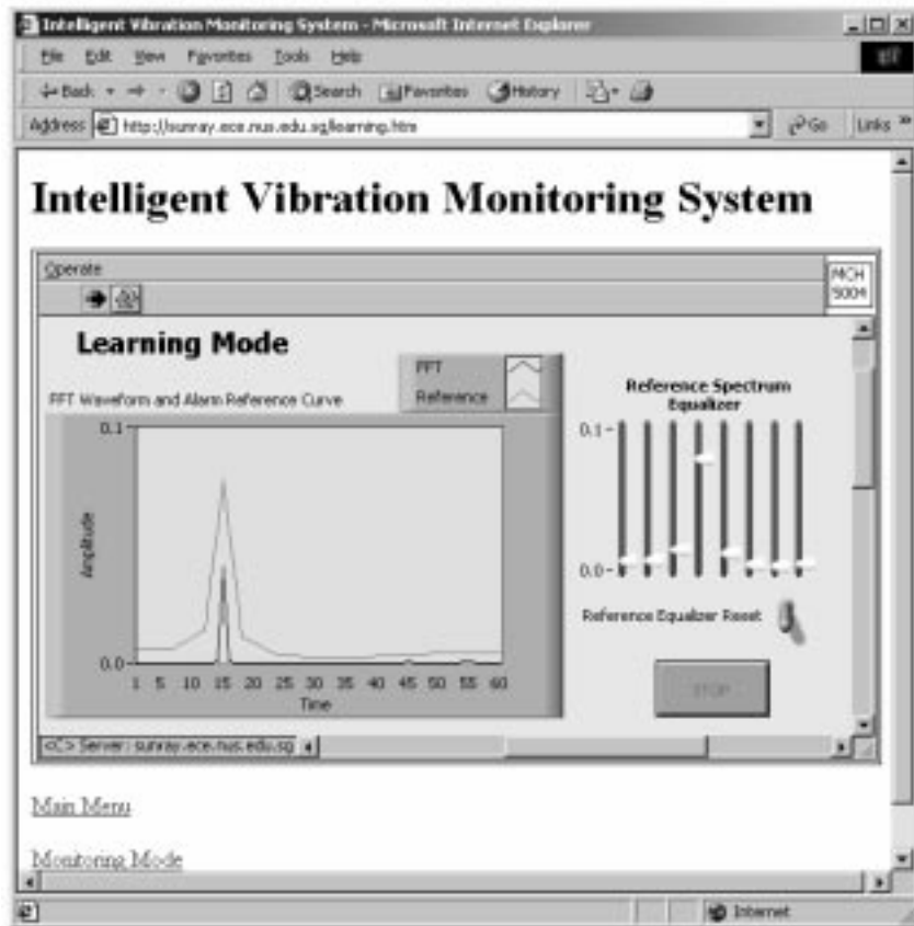
Fig. 8. Snapshot of the interface when the system is in the learning mode with the shaker receiving a 15 Hz sinusoidal signal.
