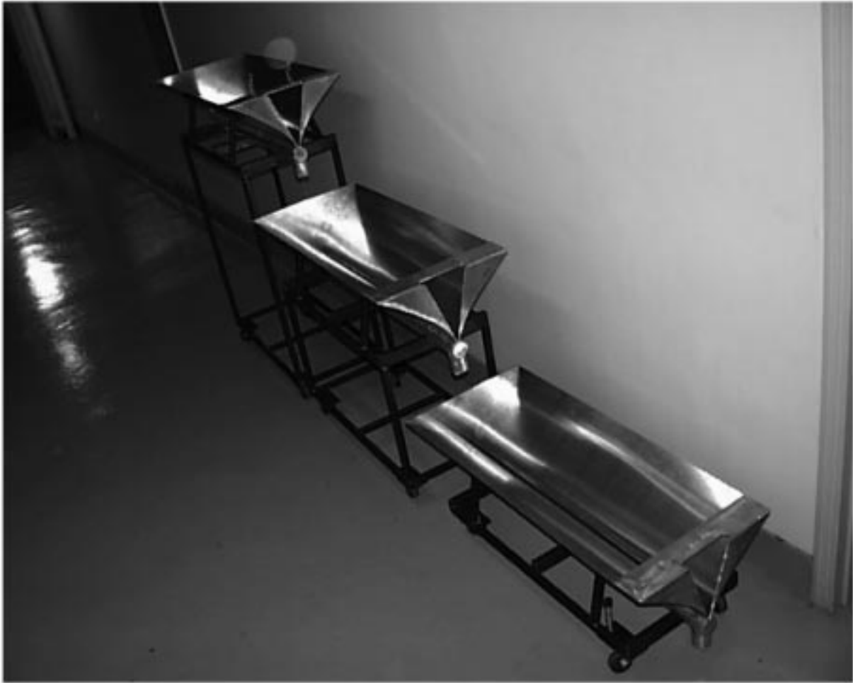
Fig. 6. The cascade of linear reservoirs (weir plates not installed).
