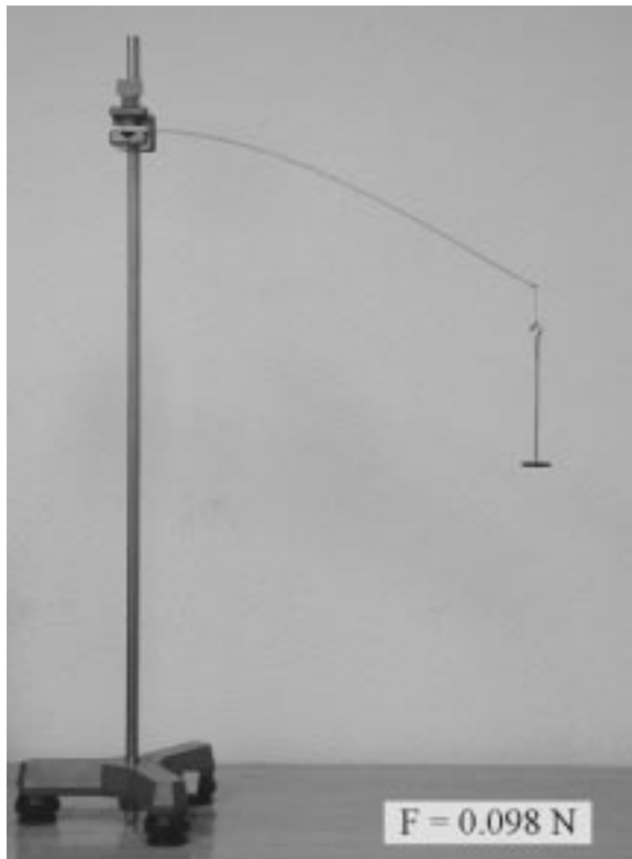
Fig. 8. Photograph of the experimental elastic curve for F=0.098 N.
