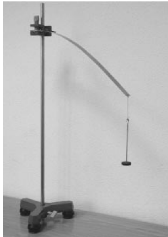
Fig. 1. Photograph of a cantilever beam loaded with an external vertical concentrated load at the free end and a distributed load (its own weight).
