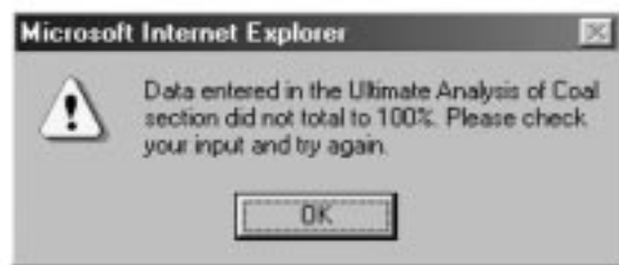
Fig. 3. Developed computer-assisted program user's interface: (a) interactive computer program for user data input and (b) activated warning dialogue boxes to prompt the user for input data errors.
