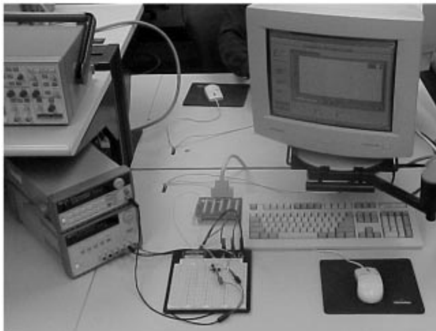
Fig. 2. Hardware setup of the integrated simulation/measurement tool used for frequency response testing.
