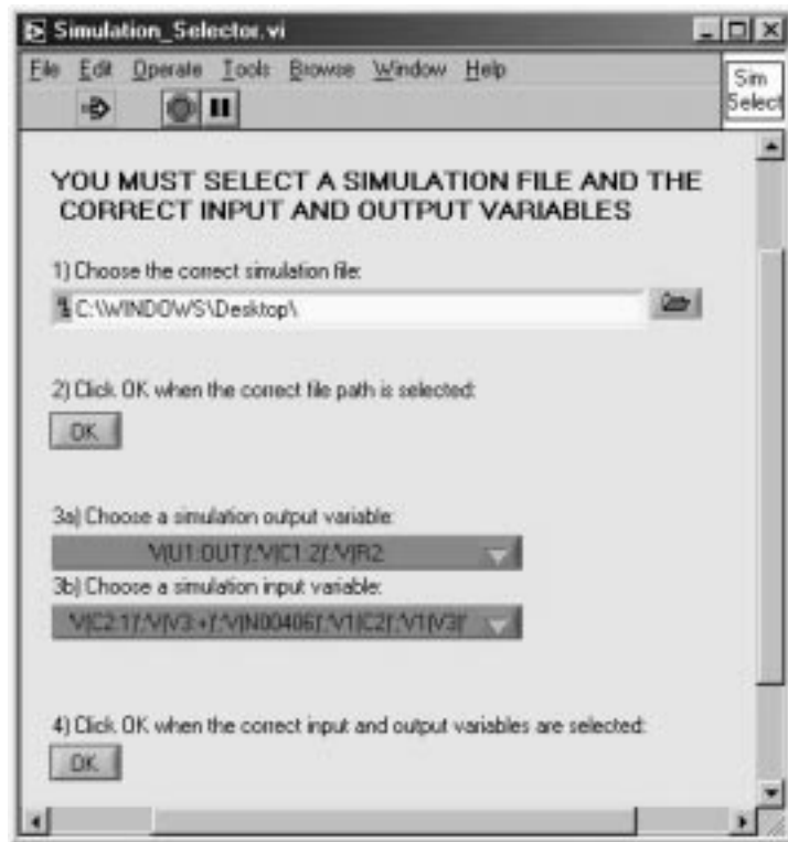
Fig. 4. The LabVIEW simulation import interface.
