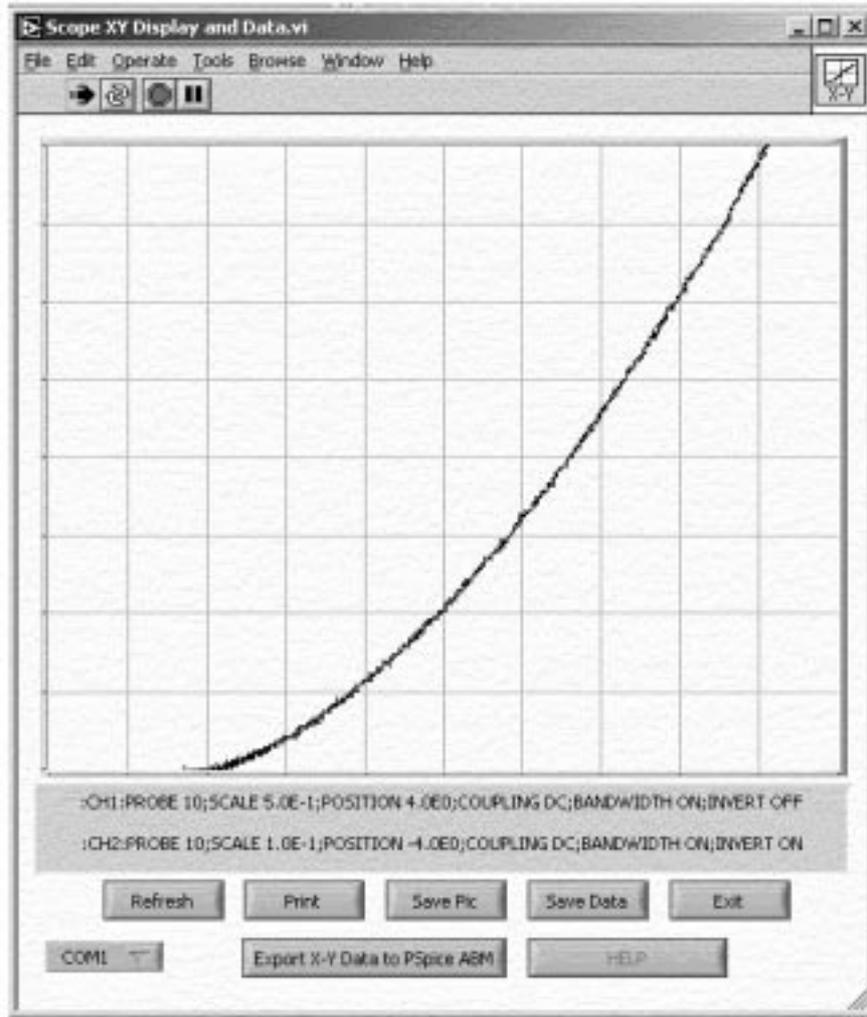
Fig. 1. Front panel of XY data and display VI.
