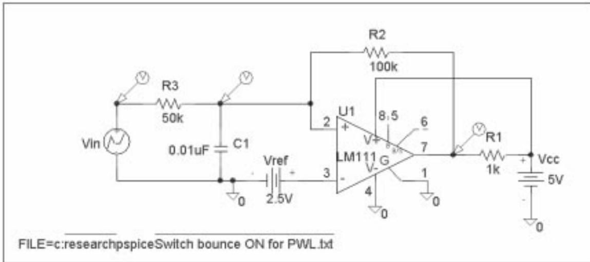
Fig. 8. PSpice switch de-bounce test circuit.
