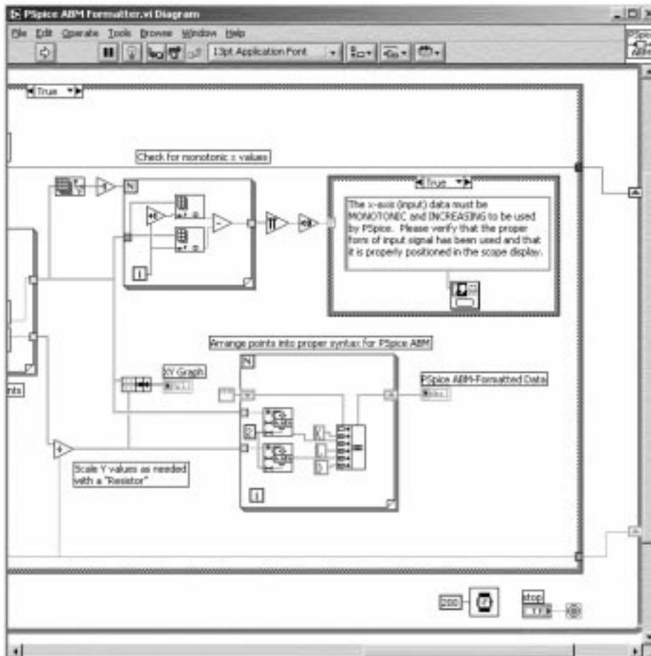
Fig. 3. Portion of PSpice ABM formatter VI diagram showing syntax formatting.
