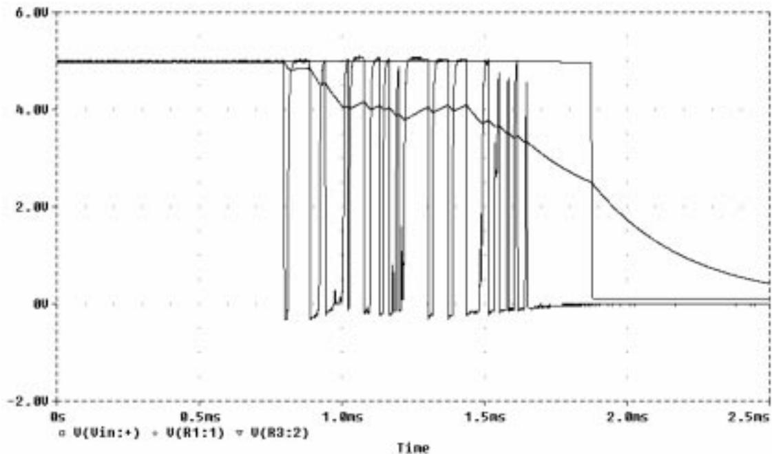
Fig. 9. PSpice (probe) switch de-bounce circuit simulation waveforms.
