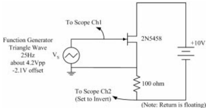
Fig. 6. Test circuit used to measure JFET transconductance.
