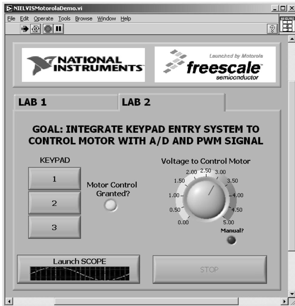
Fig. 2. Motor control front panel.
