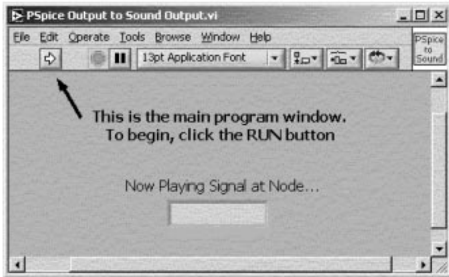
Fig. 7. LabVIEW front panel of the PSpice Output to Sound Output VI.
