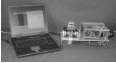
Fig. 13. Photograph of the final prototype. The compartment for the controller has been kept transparent. On the left side of the prototype, the sample holder with the stepper motor and the sample compartments can be seen.
