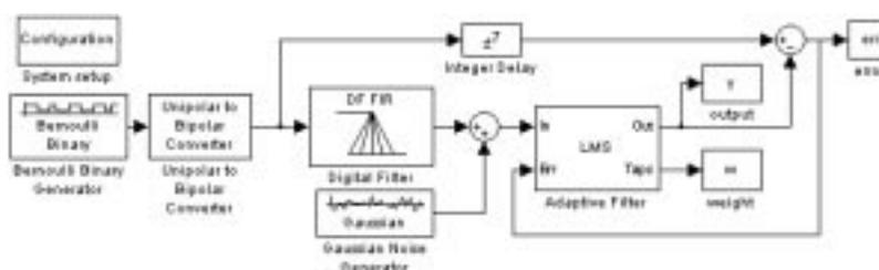
Fig. 2. LMS adaptive filter for channel equalizer.
