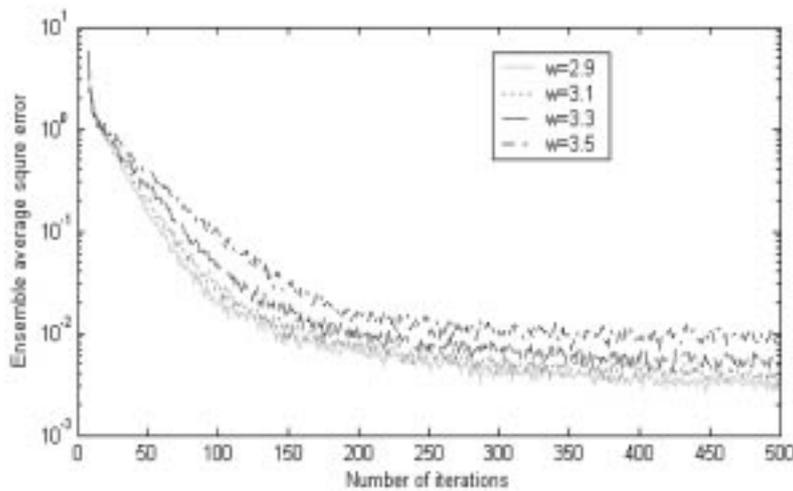
Fig. 6. GAL learning curves for  $\mu = 0.5$ . It is apparent that the learning curves are not strongly affected by the parameter  $W$ .
