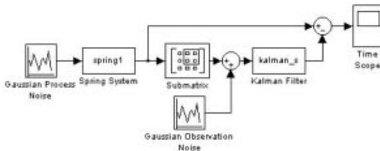
Fig. 8. The Linear Kalman Filter with the mass-spring system. Both the spring system and Kalman filter are implemented as MatLab S-functions.
