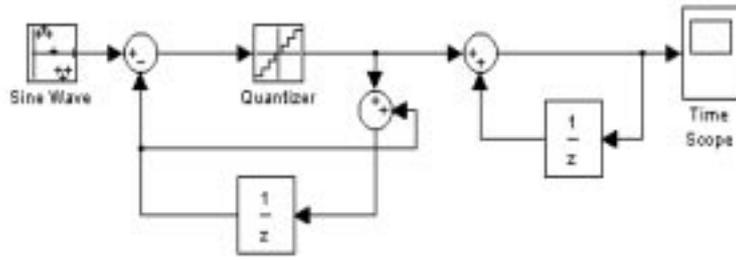
Fig. 7. The non-adaptive DPCM coder and decoder using a sine-wave source. The unit delay in the encoder can be replaced by an adaptive filter in order to test other algorithms.
