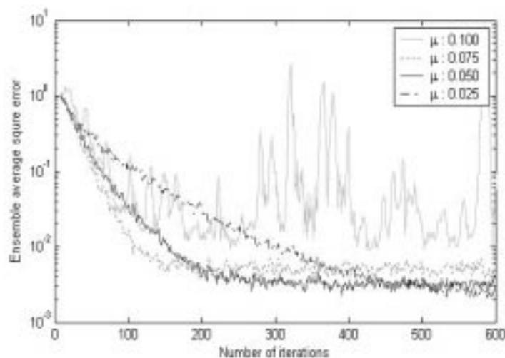
Fig. 4. LMS learning curves for  $W = 3.1$  averaged over 200 trials. In this case, it can be seen in addition to determining convergence speed,  $\mu$  also determines whether convergence occurs at all.
