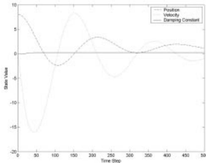
Fig. 9. State values versus time for the UKF filter. For even small mismatches in the model process noise, the damping constant state parameter may not converge.
