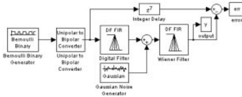
Fig. 1. Wiener filter for channel equalizer.
