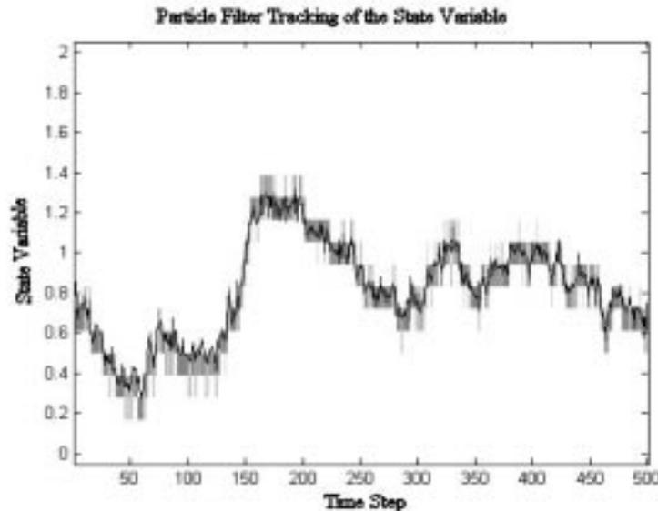
Fig. 11. State tracking using a particle filter. The particles are distributed around the state variable. The solid line shows the actual channel state and the gray squares show the distribution of the particles.
