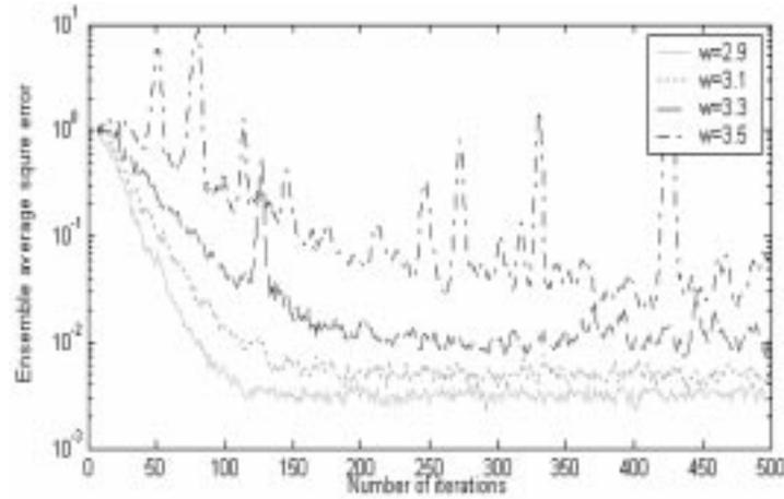
Fig. 3. LMS learning curves for  $\mu = 0.075$  averaged over 200 trials. As can be seen here, the convergence depends on the value of  $W$ .
