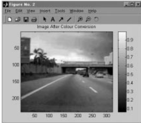
Fig. 4. Intensity (V) image in the HSV colour space.
