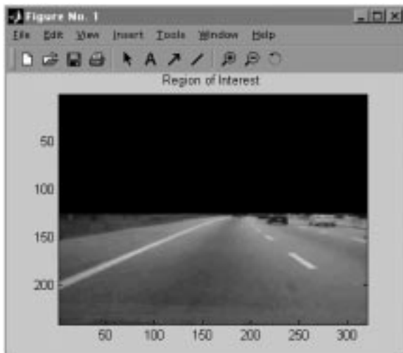
Fig. 5a. Road surface as the object/region of interest. Other objects/background are converted to black (0).
