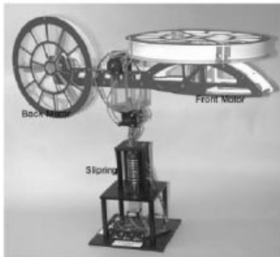
Fig. 1. The 2DOF helicopter apparatus.
