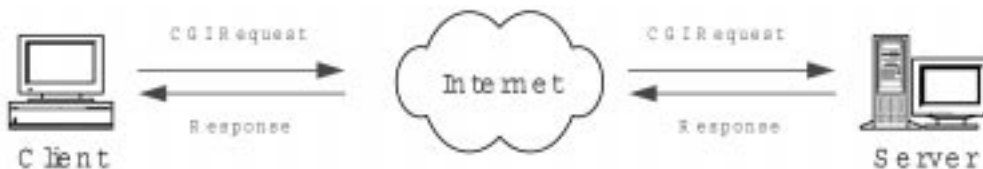
Fig. 3. A typical CGI connection.
