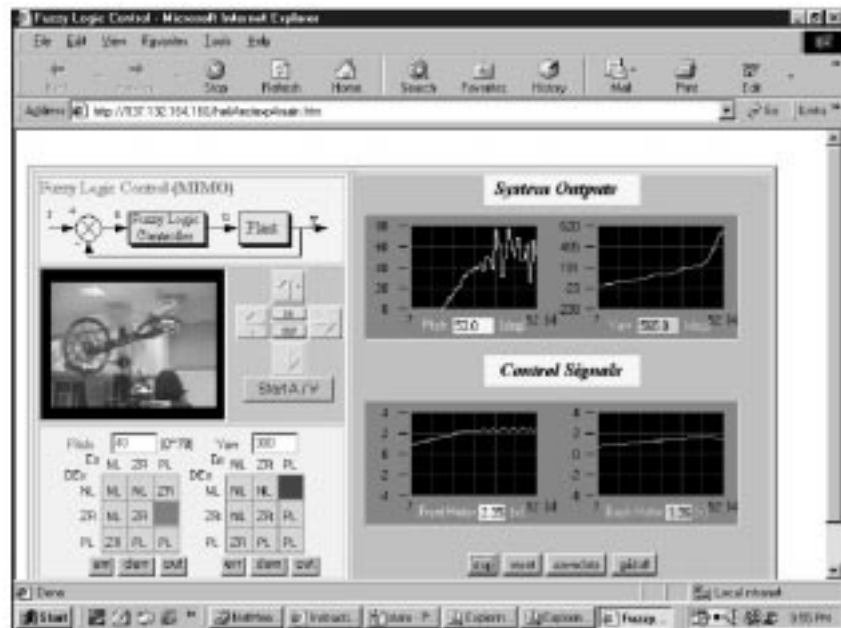
Fig. 18. Interface of fuzzy control in the web-based laboratory.
