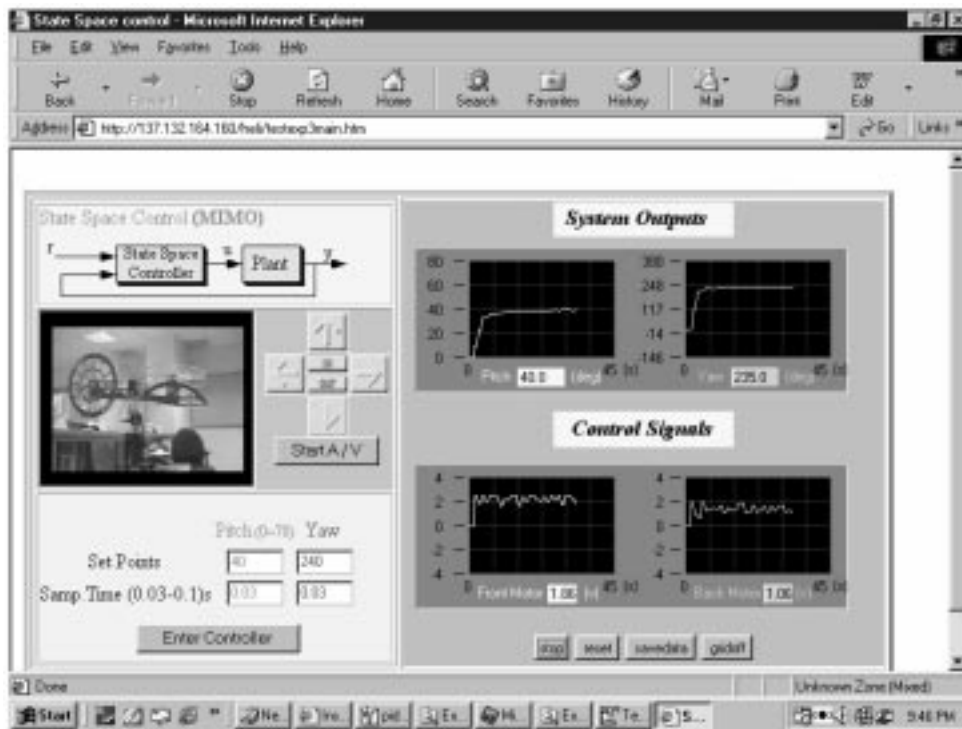
Fig. 14. Interface of state space control in the web-based laboratory.
