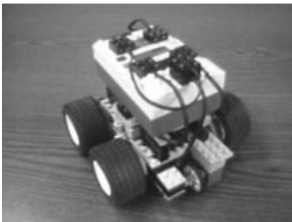
Fig. 4. The rotation sensor (encoder) is turned by the trailing wheel on the Lego MindStorms robot being used for the straight line example.
