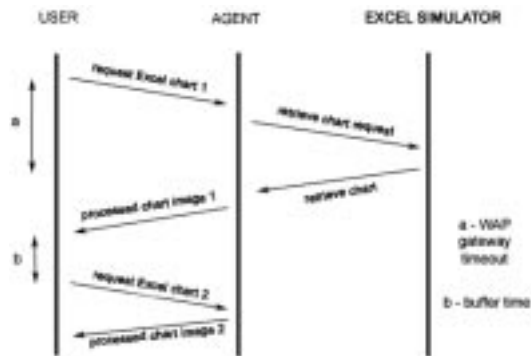
Fig. 17. Buffer. It is a small WML code downloaded into the handheld mobile device during transactions. It re-establishes the connection between the handheld mobile devices and the agent when the timeout takes place.
