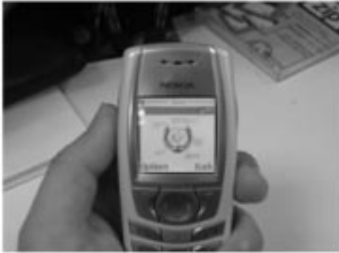
Fig. 1. PowerPoint viewing. When the user accesses the server that hosts the PowerPoint file, the application on the server automatically converts the file to an image file.
