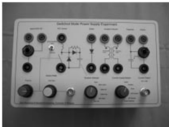
Fig. 7. Front panel of the custom-made DC-DC power electronic converter apparatus.
