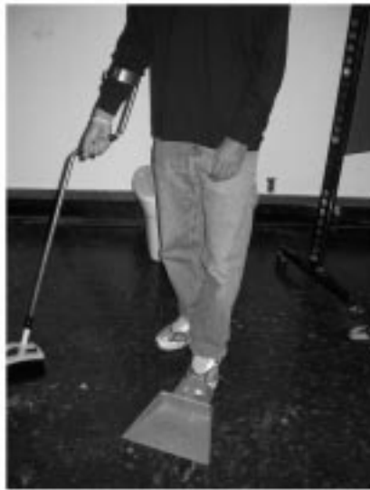
Fig. 3. (a) A system for transport and filtration to assist carrying the heavy weight as well as purify drinking water; by Team 2. (b) Broom and dustpan to minimize bending and holding requirements for users with back problems and limited hand-arm strength by Team Touche.
