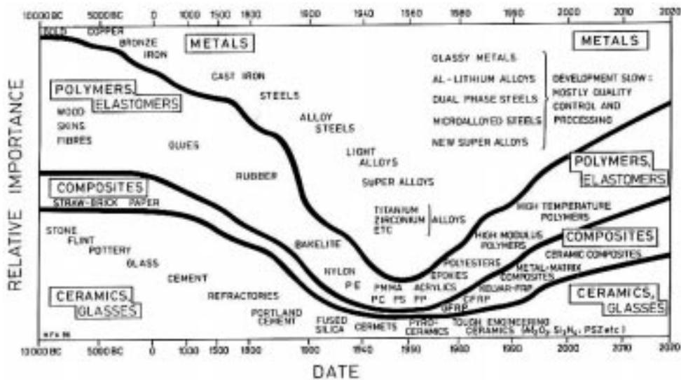
Fig. 5. Ashby's time-line [3] for the development of structural materials from the dawn of agriculture to the present day and beyond (but note the absence of functional materials for modern electronic and electro-optic applications).
