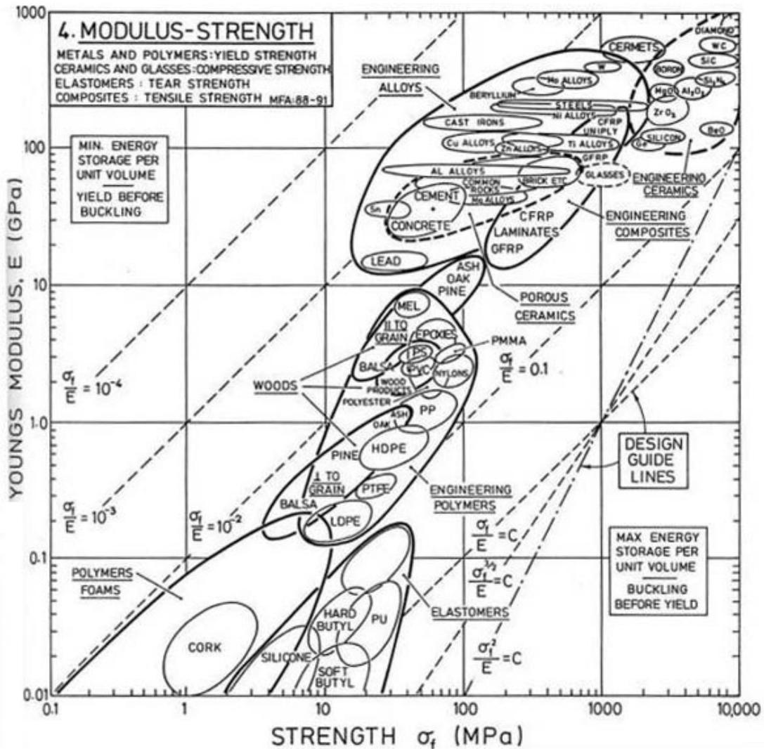
Fig. 4. An Ashby data summary [3] showing the relation between strength and elastic modulus for different classes of engineering materials.
