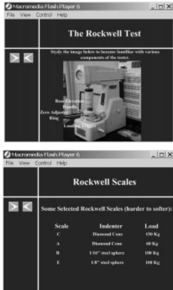
Fig. 2. The Rockwell hardness tester: (a) its components and (b) various scales identifying the type of indenter and the amount of load needed.
