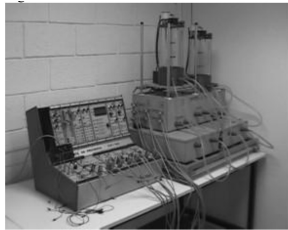
Fig. 3. Real plant with interconnected tanks.
