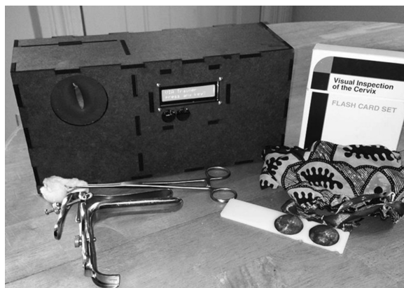
Fig. 3. Early-stage prototype of the Visualize trainer. The box-trainer (shown) allows students and midwives to practice inserting a speculum and swabbing the cervix, inspect several custom dual image tabs (shown), and diagnose and receive feedback through a built-in LCD screen.
