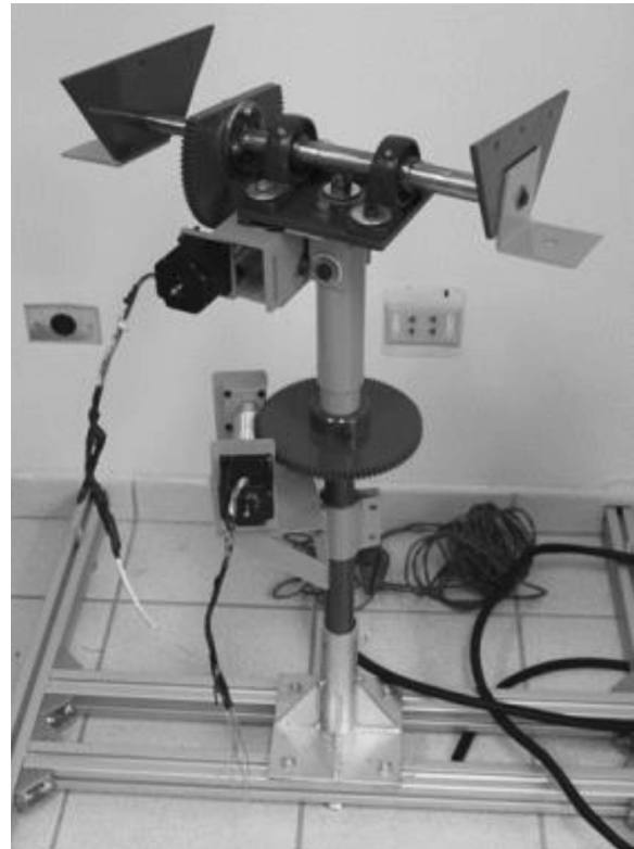
Fig. 5. Final implementation of the heliostat based on CAD (see section 2). The system was manufactured by students in campus laboratories.
