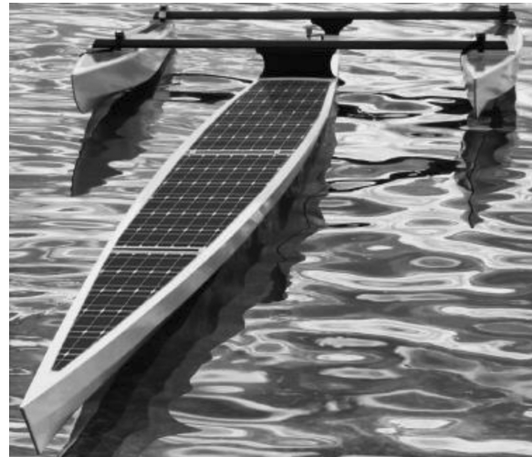
Fig. 1. Prototype of a manned auto embarkation, fed through solar energy.
