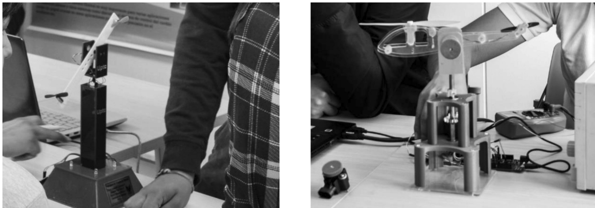
Fig. 4. Small prototypes of 2DOF helicopters comprised of two mini propellers, main and tail rotor, respectively; a) it is an ingenious model commanded by an App developed in Android (left) facilitating the interaction with the user, b) it corresponds to a prototype designed with striking shape for STEM education in K-12 courses (right).
