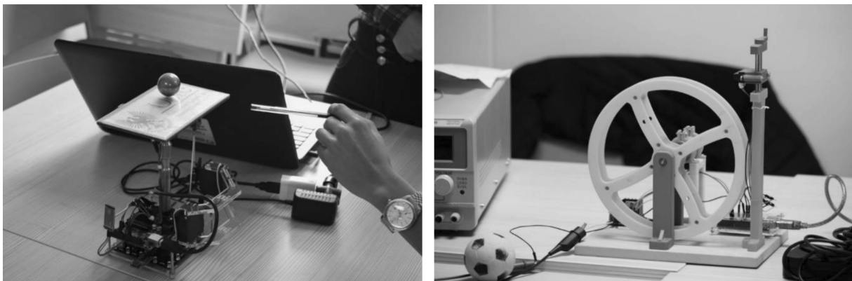
Fig. 2. (a) Small prototype of ball and plate comprised by a piezo-resistive flat and two servomotors, its structure was made in acrylic (left), (b) Small prototype of ball and wheel, its structure was made by using 3D printing (right).
