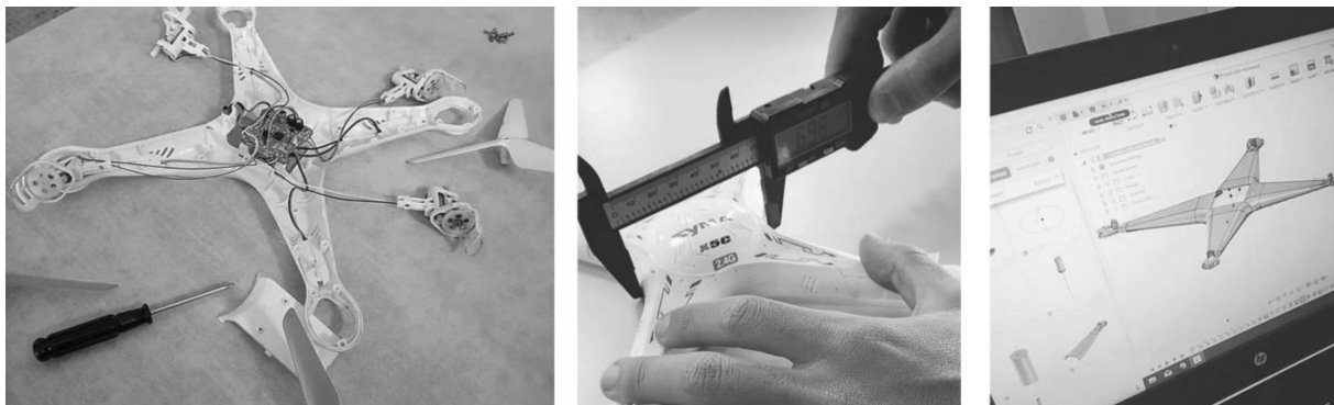
Fig. 1. Processes for graphic simulation of a drone: disassembly, measurement and digital modeling.
