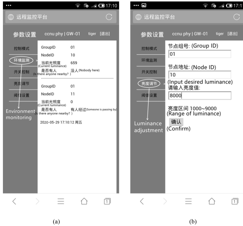
Fig. 9. Web remote monitoring UI of Smart Streetlights on an Android phone: (a) environment monitoring, (b) luminance adjustment.
