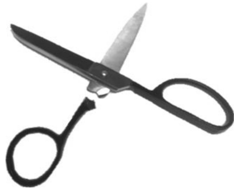
Fig. 1. Failed crafting shears used for a PjBL case-study.
